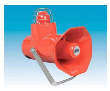
This range of beacon/sounder units, intended for use in potentially explosive gas and dust atmospheres, has a power rating of up to 10 watts (sounder) and 10 joules (beacon) and is suitable for use in the harsh environmental conditions found offshore and onshore in the oil, gas and petrochemical industries.
